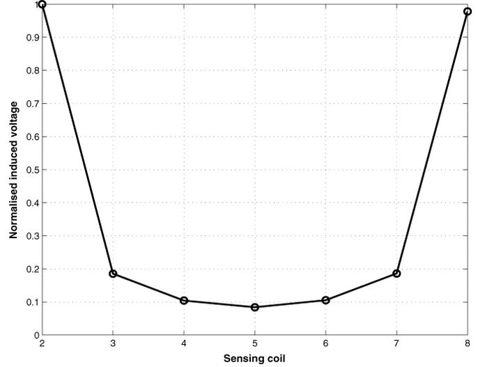
Fig. 2. Normalized induced voltage in coils 2–8 when the coil 1 is excited.
