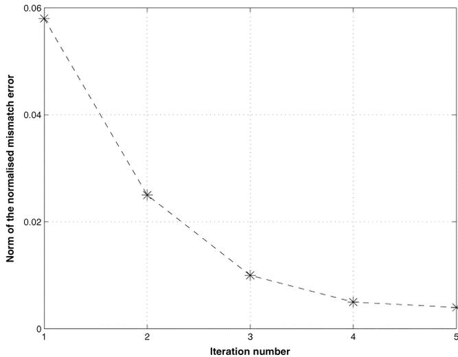
Fig. 7. Norm of the error between measured and simulated voltage (voltages are normalized to the voltage of free space).
