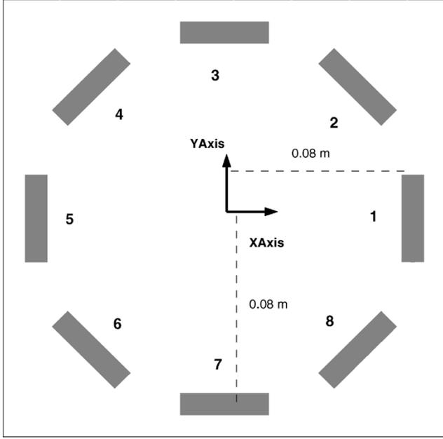
Fig. 1. Excitation and sensing coils, view from top.
