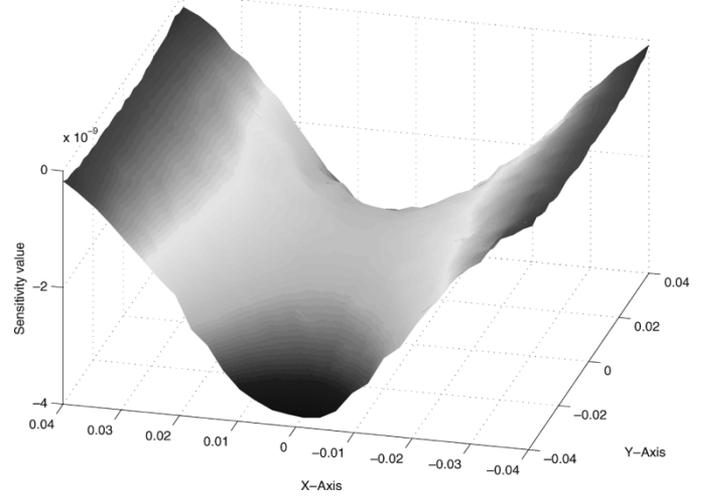
Fig. 3. Sensitivity plot for coils 1, 5 as excitation and sensing coils in plane  $Z = 0$ .
