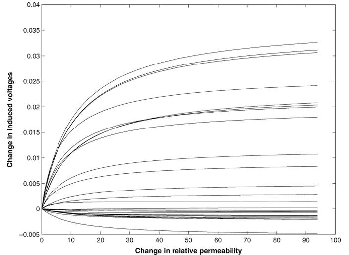
Fig. 8. Change in induced voltages (normalized to the voltage for free space) due to perturbation of permeability of a spherical object. Note the validity of a linear approximation for small changes and saturation for high changes.
