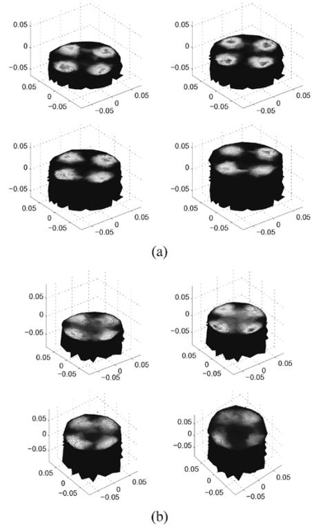
Fig. 6. Reconstruction of the test phantom in (a) can be seen in (b); the image is for different  $Z$  level of cylinder C1. (a) True object, four inclusions object with permeability 50. (b) Reconstruction of the object in (a).
